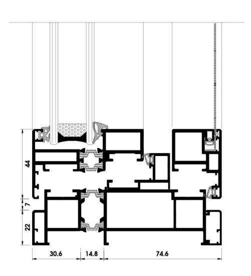
The sash levels with glass bead and frame to form a unified outlook, which is call "hidden sash". It is an application of the symmetry beauty in windows and doors.
